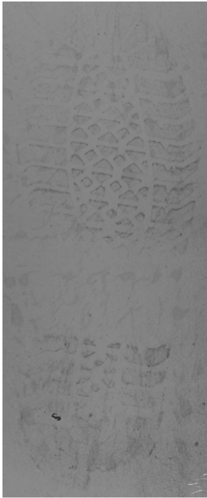
FIG. 2—Footwear impression lifted by the Electrostatic Detection Apparatus 2 from a sheet of paper originally placed on a nylon carpet when the footwear impression was made.
